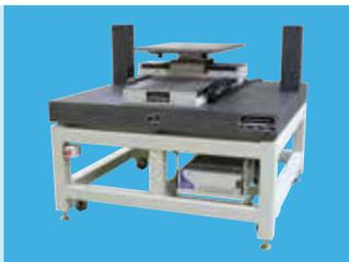
曝光直寫式曝光 (無光罩曝光)
