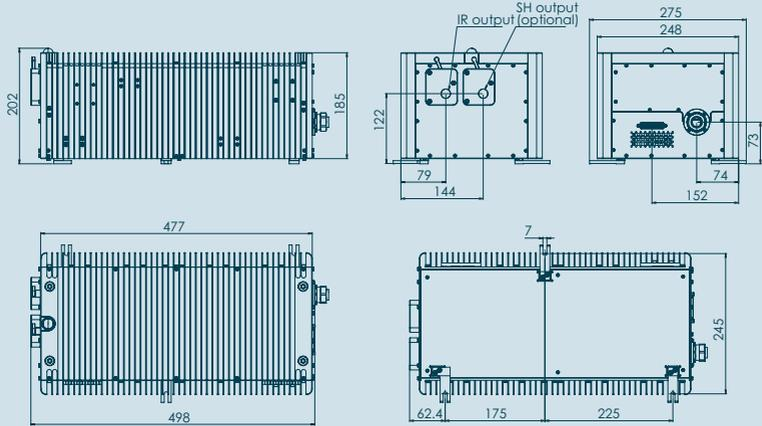
Drawing of Indylit 10 laser head (in mm)
